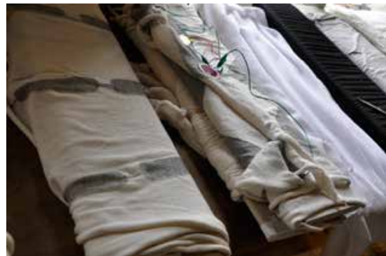
Figure 1. Smart-textiles capable of measuring stretch as semi-finished products developed in STS project, hooked up to a Lilypad Arduino microcontroller
