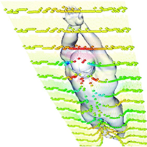
Figure 5. Pulsed waterflow pathlines over the body coloured by static pressure. <http://www.biomimicryinstitute.org>
