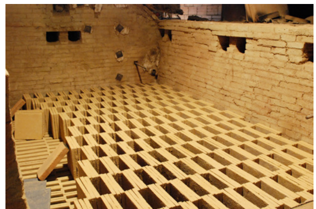
Handmade bricks mounted in the oven for firing. (Quart, Spain)
