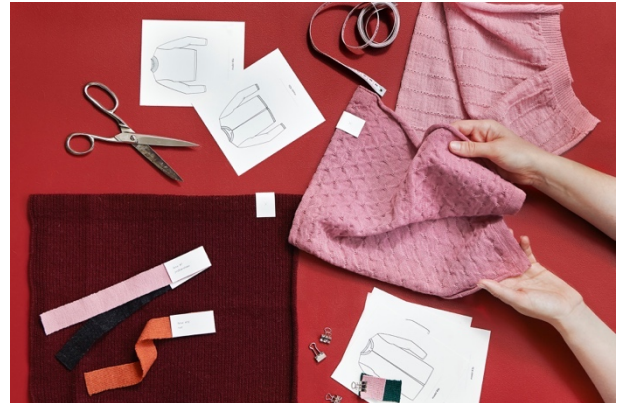
Figure 8: Examples of the knitted prototypes, colour samples and working drawings of jumper style.
