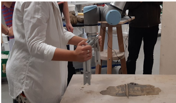
Figure 3. The movement of the robot is recorded by manually moving the attached tool.
