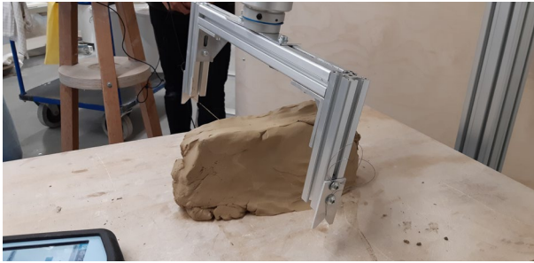
Figure 6. The execution of the cut by the robot arm through a lump of clay.
