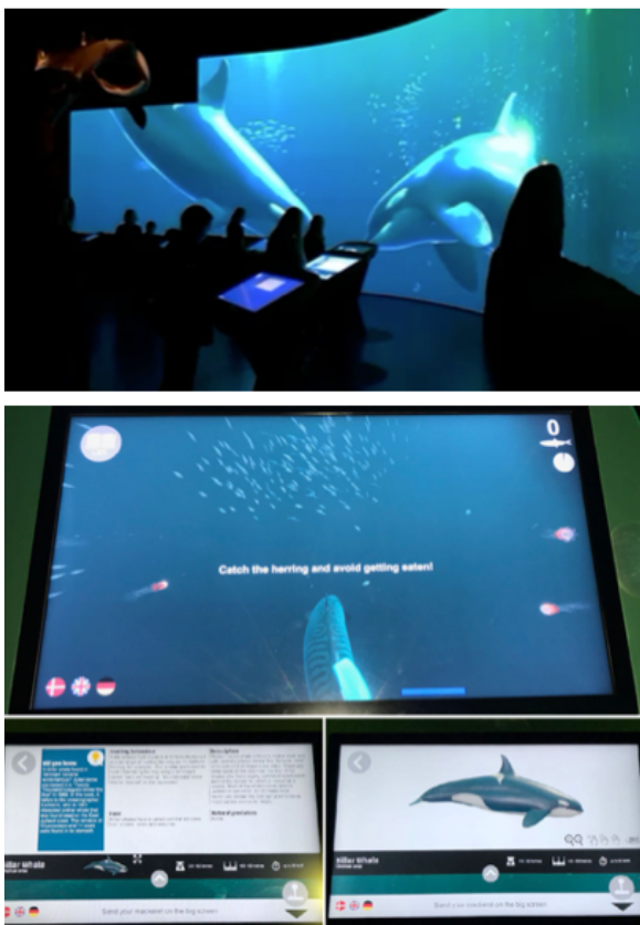
Figure 3: Images of the 'Big Ocean Window' installation. The big 100 m 2 interactive LED screen (top) is interacted with through eight big touch screens (middle) which besides the game-based mackerel also includes a lexicon feature (bottom).
