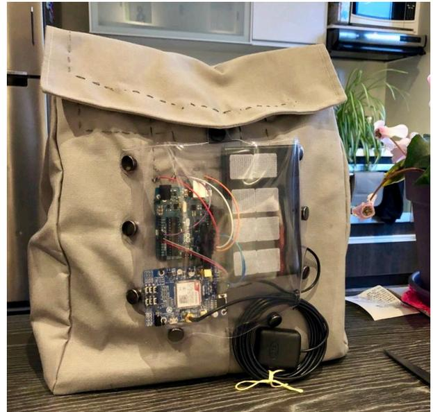
Figure 5: The final iteration of *La Encomienda*. In the front, the textile bag has a plastic pocket that contains a microcontroller prototyping board, a cellular module, an antenna and a packet of AA batteries.
