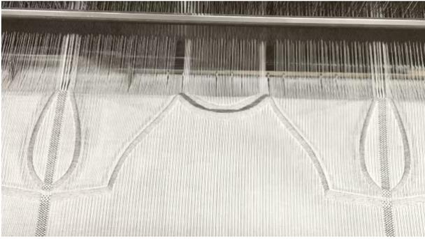
Figure 7: Video showing the weaving and cutting for the tshirt.
