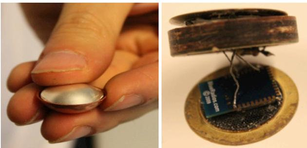
Figure 4: a) Prototype button crafted out of copper and silver, b) The electronics hosted inside a previous version of the ‘copper and silver button’. Conductive thread used to connect the metal surfaces with the BLE module.
