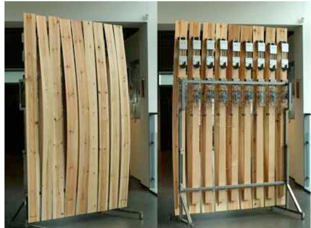
Figure 4 Nine PLANKS placed on a stand shown from the front and the back with the visible computational layer.
