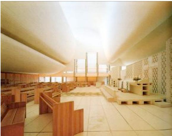
Figure 1 Bagsværd Church, designed by Jørn Utzon is an example of how the regulation of sound have influenced the form of the room especially the ceiling. Photo by: Søren Kuhn
