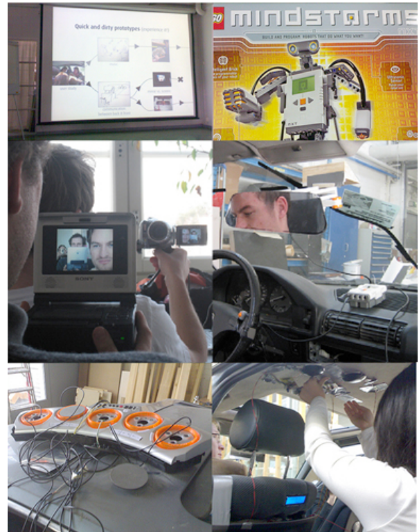
Picture 6. Up: from user study to concepts and Mindstorms. Middle: Gaining empathic insight by using a small LCD screen and video camera as a proxy for a mirror and iterating the interactive mirror concept in-situ with Mindstorms in Mirror . Down: hacking toys in Car Body and testing Bugbugs .
