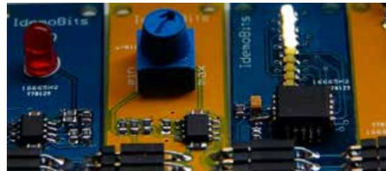
Figure 1: IdemoBits with sensors and outputs
