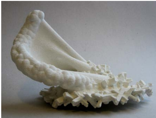
Figure 6: The digital shape is shown as created in ceramics by the use of a 3D powder printer from ZCorp
