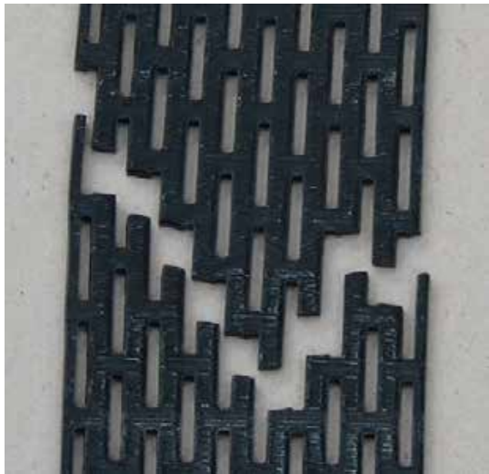
Figure 10. Typical parallel sample breakage
