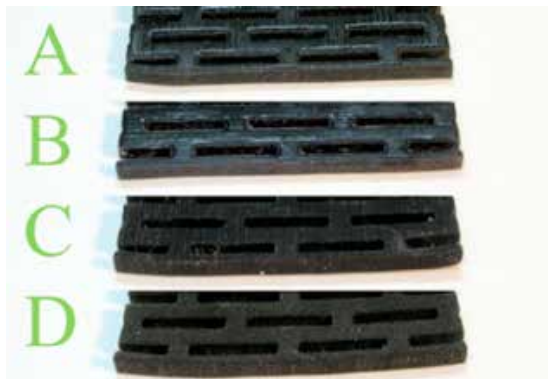
Figure 4. Outcome of four different print directions on orthogonally patterned pieces
