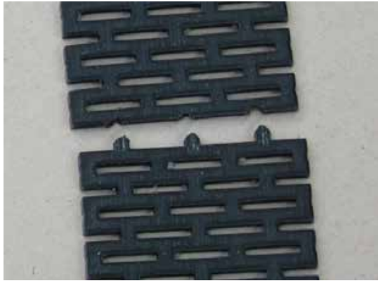
Figure 9. Typical orthogonal breakage
