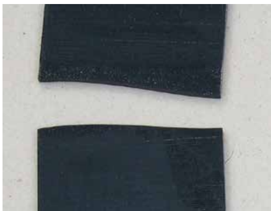
Figure 11. Typical plain sample breakage
