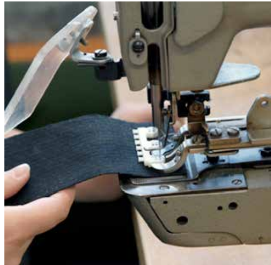
Figure 14. Attaching the connector with a machine
