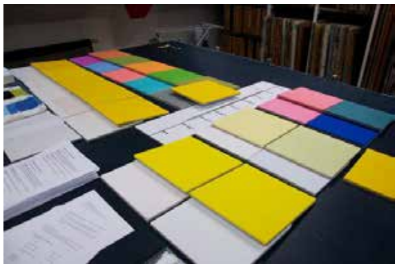
Figure 1. shows color-swatches made with textile pigment pastes to demonstrate the varying colors of leuco dye-based thermochromic inks at different temperatures.
