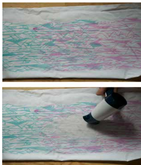
Figure 8. From top to bottom: sample of prints made with the turquoise and magenta inks with activation temperature 27°C at ambient temperature (20°C) and the effect of heating the printed fabric. Work by Bachelor Student Cecilia Krook, thermochromic workshop, 2012.
