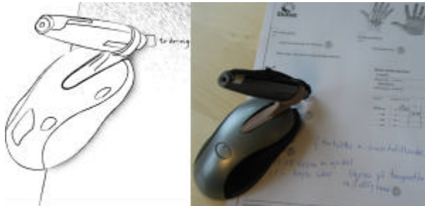
Figure 5: Mouse++, sketch and first prototype.
