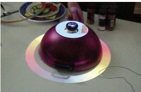
Figure 3: The projected color ring shows the temperature setting of the "Tada." The color on the lid shows the temperature of the food as it heats.
